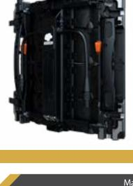
Pixel Pitch: 2.6, 3.9 and 5.9mm Pixels per Display: 176x176/128x128/84x84 LED Source: SMD 2121 RGB LEDs (SMD 1515 for EVHD 2.6) Viewable Angle: 140° H, 120° V NITs: 1,200 Nits Max Power Usage: 165W, 125W, 120W IP Rating: IP20 Tile Size: 19.7 x 19.7" Weight: 19.8, 18.7, 18.7 lbs. **Certification:** CE cETLus **Notes:** Front serviceable: lockable curve
