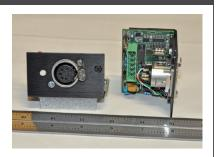
bicolor LED for status indication. Data and power distributed by a private DMX/RDM buss using screw terminal blocks. Powered by a 24VDC supply @ 38mA per module.
